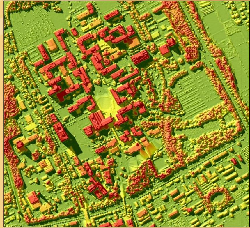
DTM and DSM generation from LIDAR data to measure terrain height and surface height (from sea level).
