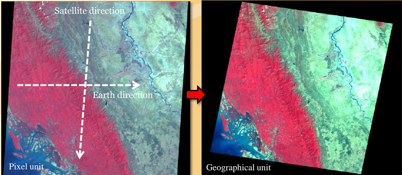
Geometric distortion due to Earth rotation.
