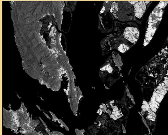
Band 5 : Mid-Infrared (1.550 ~ 1.750  $\mu\text{m}$ )
