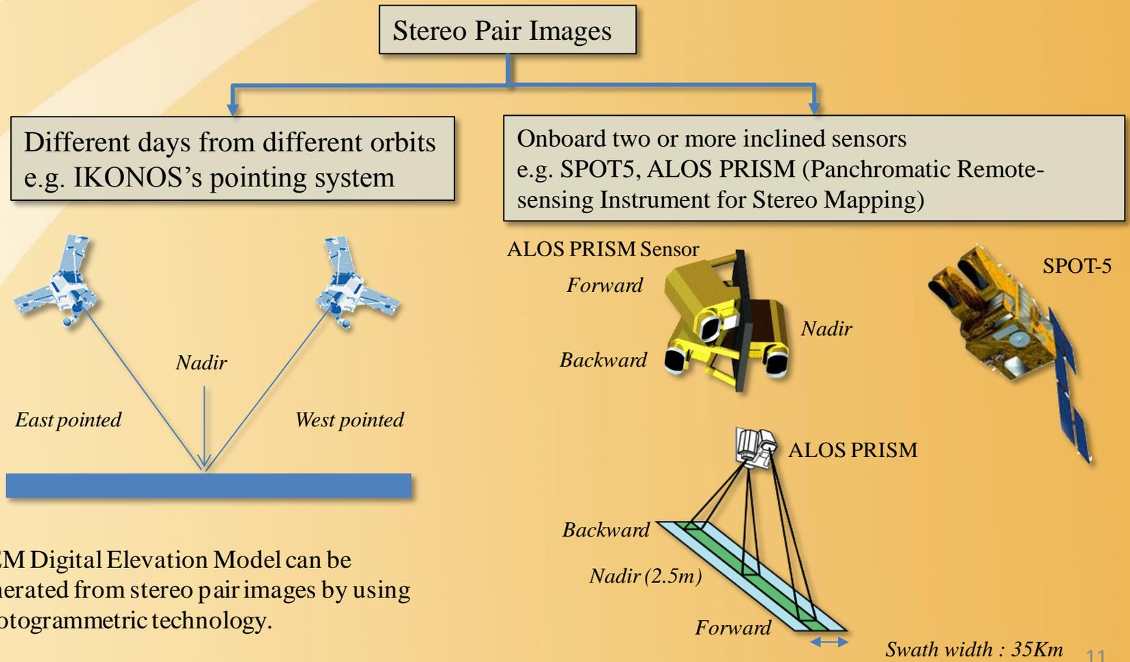
DEM Digital Elevation Model can be generated from stereo pair images by using Photogrammetric technology.
