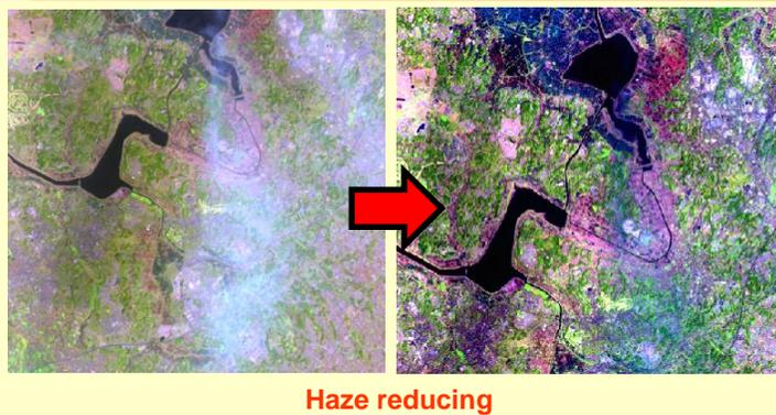
Small haze can be removed in Landsat TM/ETM.
