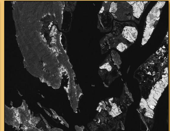
Band 7 : Mid-Infrared (2.090 ~ 2.350  $\mu\text{m}$ )
